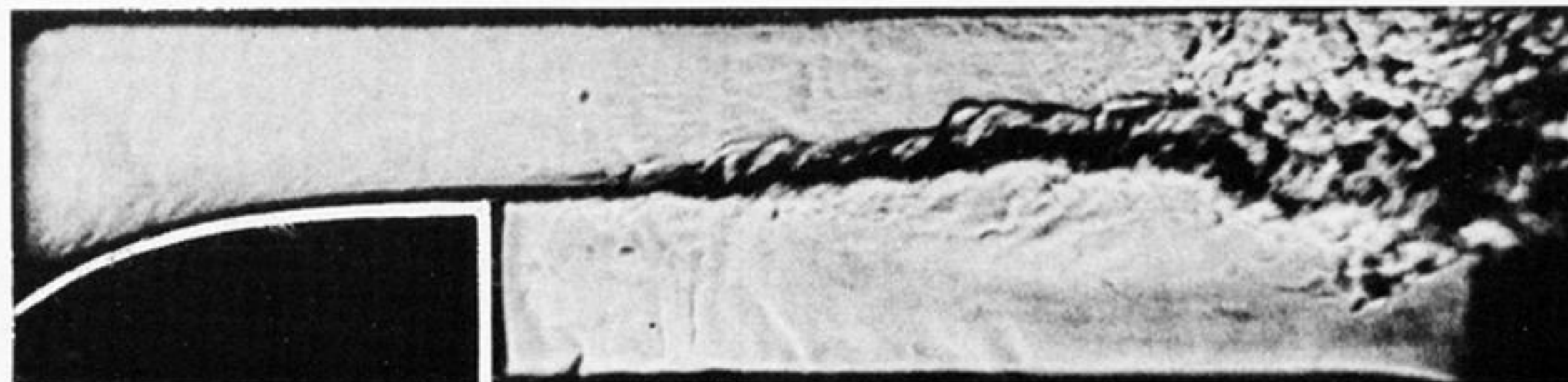
FIGURE 14. Cinematographic schlieren records of turbulent flame in a combustion tunnel. Height of channel is 5 cm. Reynolds number of flow at inlet of 5 cm is around 10^4 . Sequence is from the top at intervals of around 19 ms between frames.
